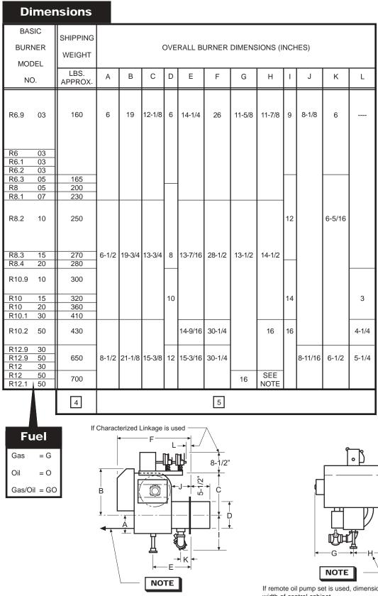
Dimension F plus burner nose length (5-1/2" standard) is required behind the burner to remove the drawer assembly.
