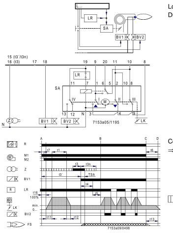
Load control with an on / off controller. During burner off times, the air damper is closed.
