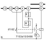
If an auxiliary contact «d1 / d2» of the fan contactor is included in the circuit as shown in the diagram, ignition and release of fuel are possible **only** when the contact is closed.
