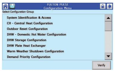
FIGURE 45 - ACCESSING CENTRAL HEAT CONFIGURATION
